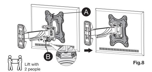
With two people, lift and hold the TV in place while tightening the bolts using the spanner supplied 9 to secure the TV.
