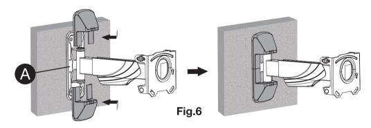
Once the bracket arm has been securely attached to the wall, place the plastic ers over the back of the bracket see Fig.6
