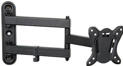
28085T Screen Size: 14-24" Max VESA: 100 x 100 Extends: up to 408mm Tilts: +3/-12° Swivels: +90/-90°
