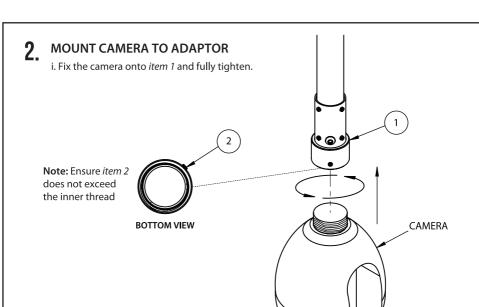
ii. Tighten *item 2* on the bottom of *item 1*, securing the camera to the adaptor.
