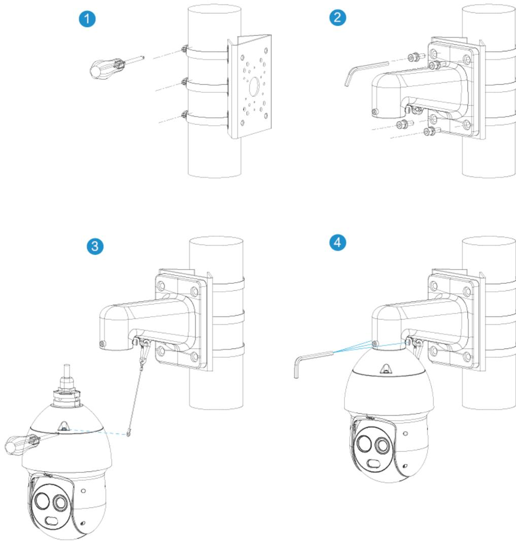
Figure 4-4 Corner-mount installation
