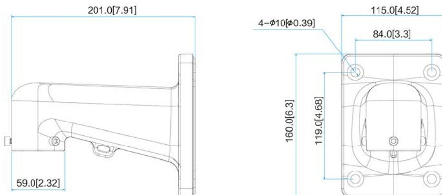
Figure 2-3 Pole-mount bracket (mm [inch])
