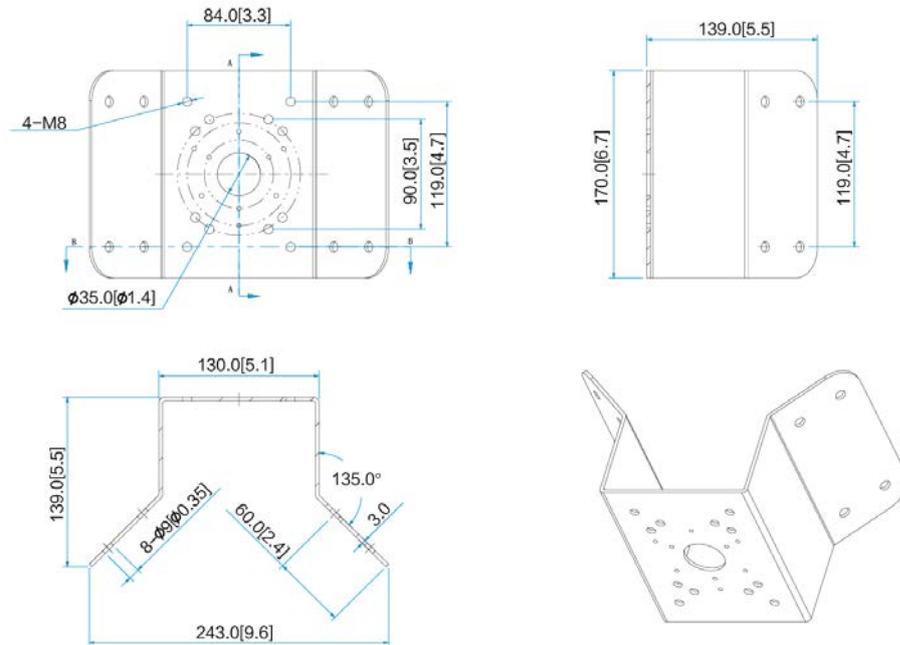
Figure 2-5 Ceiling-mount bracket (mm [inch])
