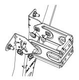
**3.** Attach Elevation Bracket (3) to Antenna Bracket (2) using 4 off M6x16 cup square screws (12) & M6 nuts (10).
