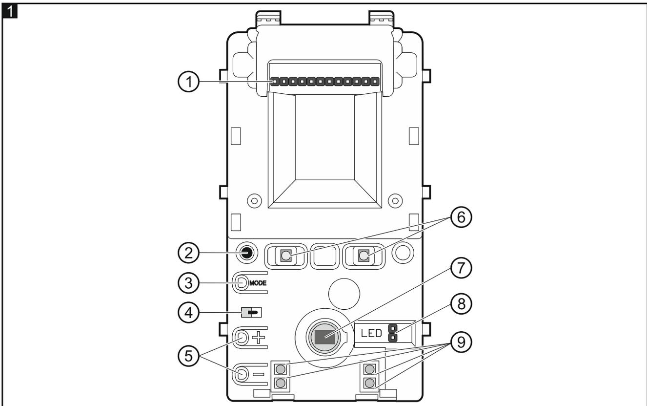
① pins for configuration of the detector outputs. Available settings are shown in the figures:
