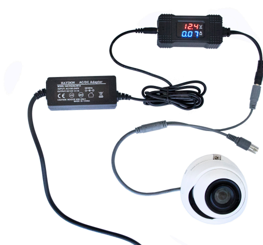
Fig 1 Shows camera current and voltage in normal mode
