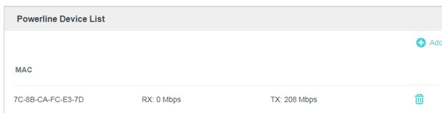
3. Click the [add](#) icon [+](#) and enter the [Powerline Key](#) of the device you want to add. The Powerline Key contains 16 capital letters, formed like XXXX-XXXX-XXXX-XXXX. It is printed on the back of the powerline device.
